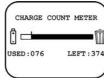
The warranty on all batteries is 12 months or 450 charge cycles, whichever is the sooner. After 420 cycles, at switch on the radio will emit a series of short tones, and on LCD models a waste bin icon will flash to alert you to the need to buy a new battery.
