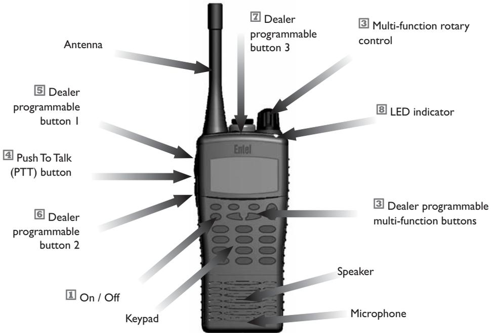
**1** On / Off button. Press to turn radio on, press and hold to turn off.
